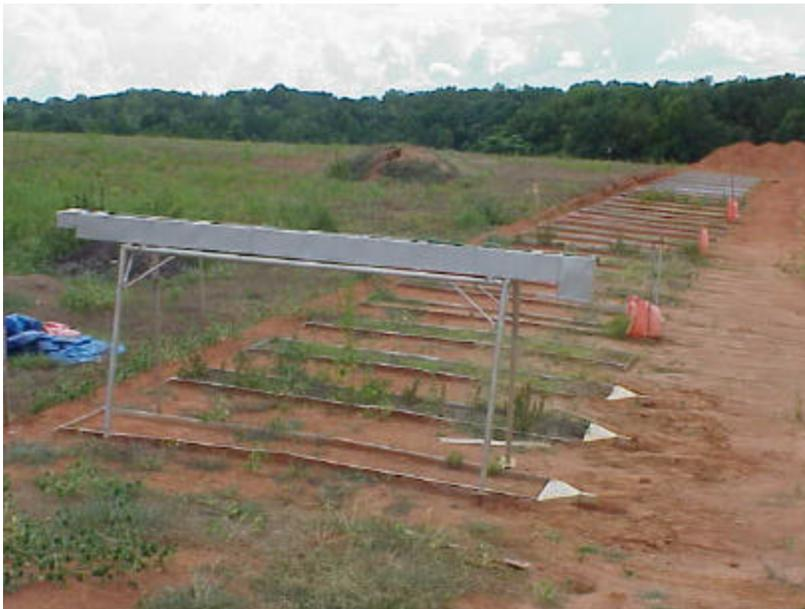
**Figure 1.4:** Experimental site layout with rainfall simulator.
