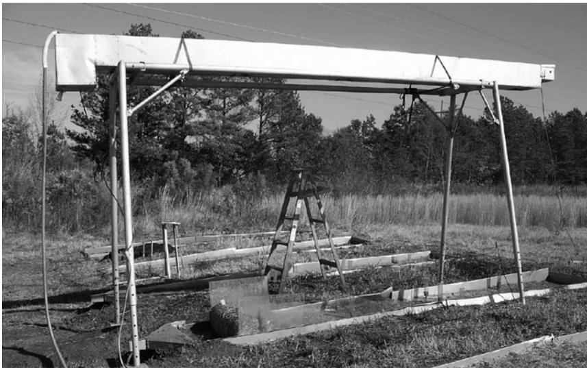
in) into the soil. To collect runoff, a removable flume was installed at the base of each plot prior to each simulated rainfall event (figure 2). To maintain the structure and integrity of the soil in the plot, a removable stainless steel border was carefully inserted at the base of each plot once the flume was removed after each storm event. The soil
