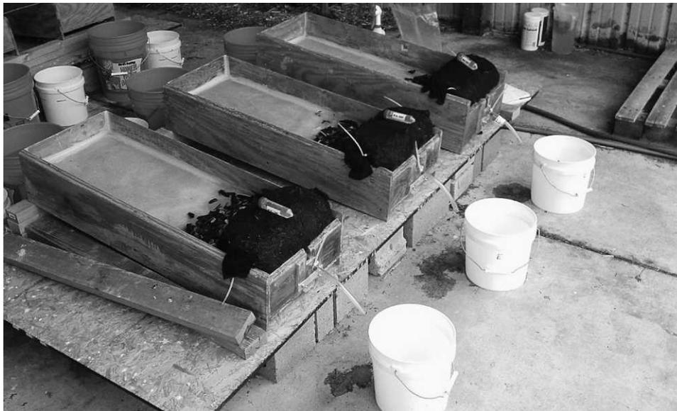
**Figure 1—Bench scale experimental set-up. Experimental box (micro-watershed) inside dimensions were 1 m length by 360 mm width by 250 mm depth. Treatments were 200 mm in diameter and 360 mm in length.**
