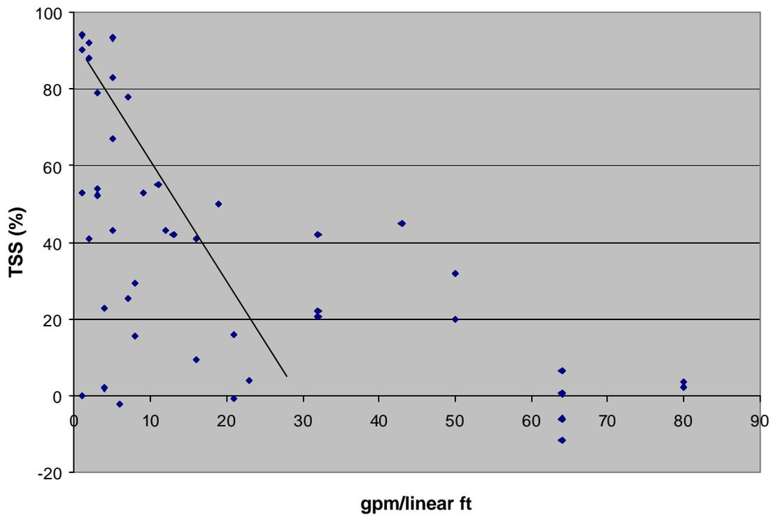
Figure 6--Hydraulic flow through rate of filter media relative to turbidity reduction in runoff.
