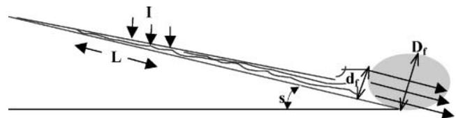
Fig. 11. Diagrammatic representation of control structure in operation and variables used to calculate water runoff rates.  $I$  = rainfall intensity,  $L$  = slope length,  $s$  = angle of slope,  $d_f$  = height of water retained by the filter perpendicular to slope,  $D_f$  = filter height or diameter.
