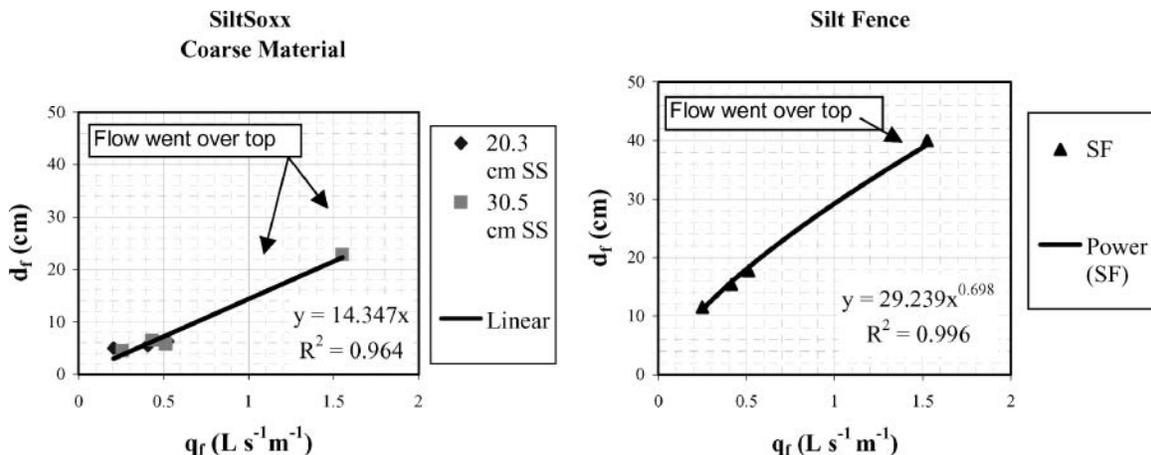
Fig. 7. Depth vs. sediment-laden water flow rate after 30 min of run time for the 20.3-cm diam. (8 in) coarse SiltSoxx (SS), 30.5-cm diam. (12 in) coarse SS, and 61.0-cm (24 in) silt fence mounted 45.7 cm (18 in) above flume bottom.
