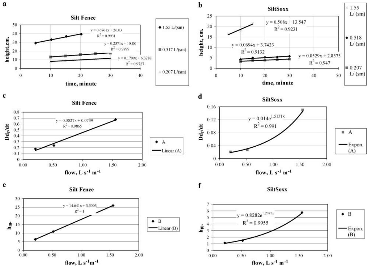
Fig. 8. (a–f) Evaluation of pond depth retained by a silt fence and SiltSoxx as a function of flow rate and time for sediment-laden water runoff.
