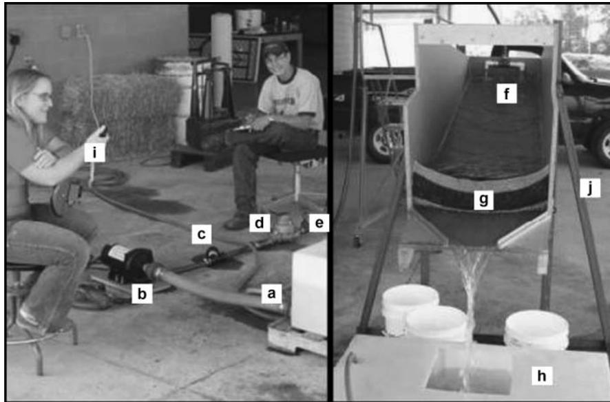
**Fig. 1.** Laboratory test setup using a flume 0.61-m width by 2.44-m length (2 by 8 ft.) to determine flow-through capacity of SiltSoxx and silt fence with clear water. (a) Outlet from supply tank, (b) pump, (c) filter, (d) flow meter, (e) valve, (f) header, (g) 20.3-cm diam. (8 in) SiltSoxx, (h) 151-L (40 gal) water tank, (i) timer, and (j) frame.
