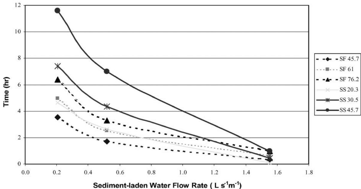
Fig. 9. Time to overtop silt fence (SF) and SiltSoxx (SS) as a function of sediment-laden water flow rate.  $\psi = 0.85$  for SF and  $0.80$  for SS.
