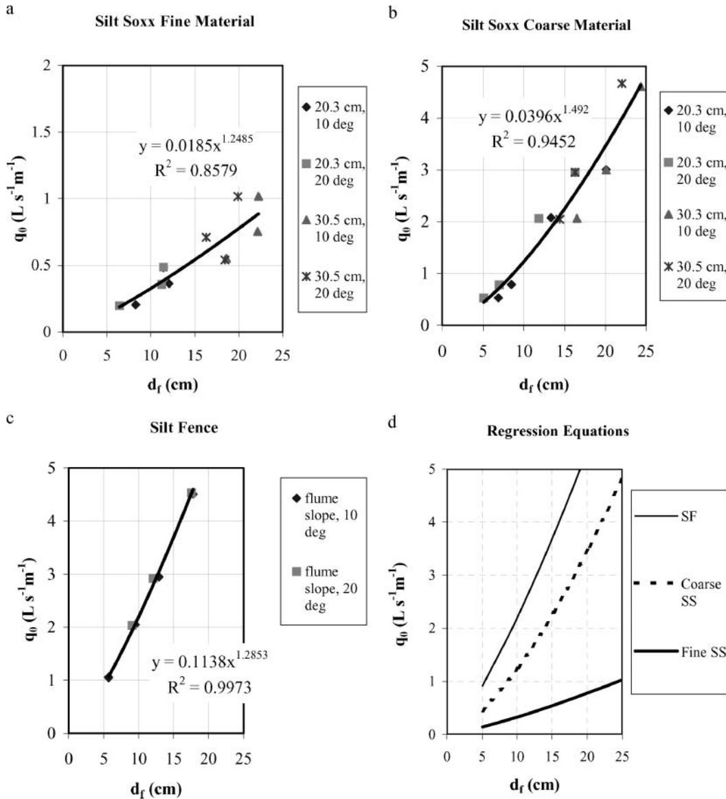
Fig. 5. Flow-through rates ( $q_0$ ) for clear water vs. ponding depth of water for: (a) SiltSoxx (SS) using fine compost (see Table 1) for both 10° and 20° slopes vs. depth, (b) SS using coarse compost (see Table 1) for both 10° and 20° slopes vs. depth, (c) silt fence (SF) for both 10° and 20° slopes vs. depth, and (d) fine SS, coarse SS, and SF using regression equations.
