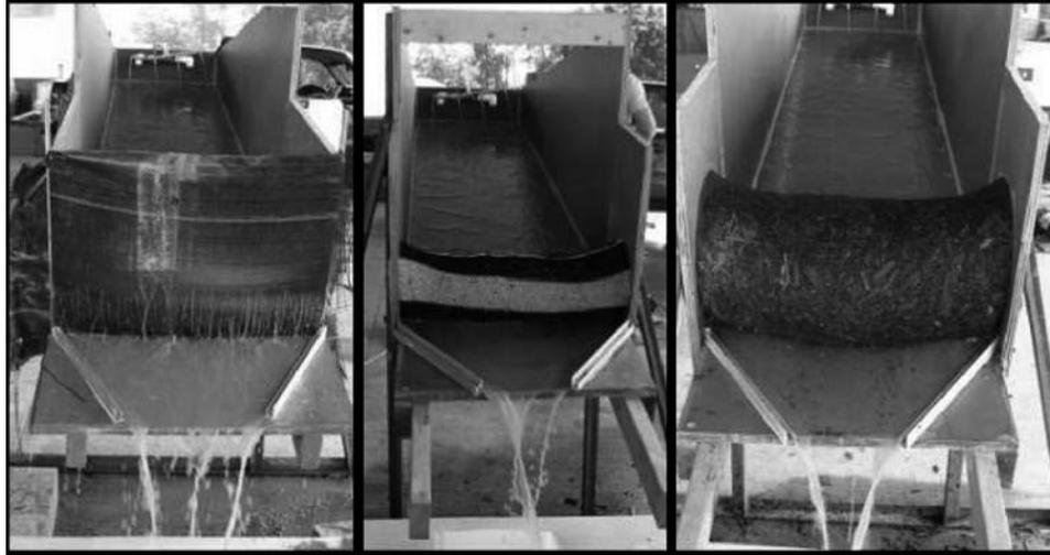
Fig. 4. Flow of sediment-laden water through sediment control devices at  $0.126 \text{ L s}^{-1}$  (2 gpm) at  $t = 10$  min. From left to right, 61.0-cm (24 in) silt fence mounted 45.7 cm (18 in) above flume bottom, 20.3-cm diam. (8 in) coarse SiltSoxx, and 30.5-cm diam. (12 in) coarse SiltSoxx.
