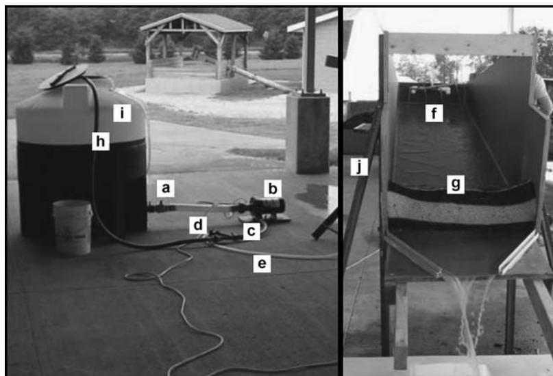
**Fig. 2.** Laboratory test setup using a flume to determine filtration and flow-through capacity of SiltSoxx and silt fence using sediment-laden water. (a) Outlet from supply tank, (b) pump, (c) Y tee, (d) valve in recirculation line, (e) delivery line, (f) header, (g) 20.3-cm diam. (8 in) SiltSoxx, (h) by-pass flow line, (i) 643-L (170 gal) cone bottom tank, and (j) frame.
