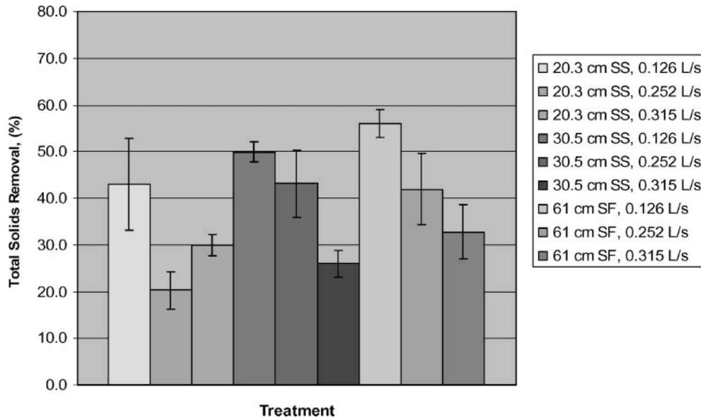
Fig. 10. Total solids removal efficiency for 20.3-cm diam. (8 in) coarse SiltSoxx (SS), 30.5-cm diam. (12 in) coarse SiltSoxx, and 61-cm (24 in) silt fence (SF) with a height of 45.7 cm (18 in) above the flume. The standard error of the means for each treatment is shown.
