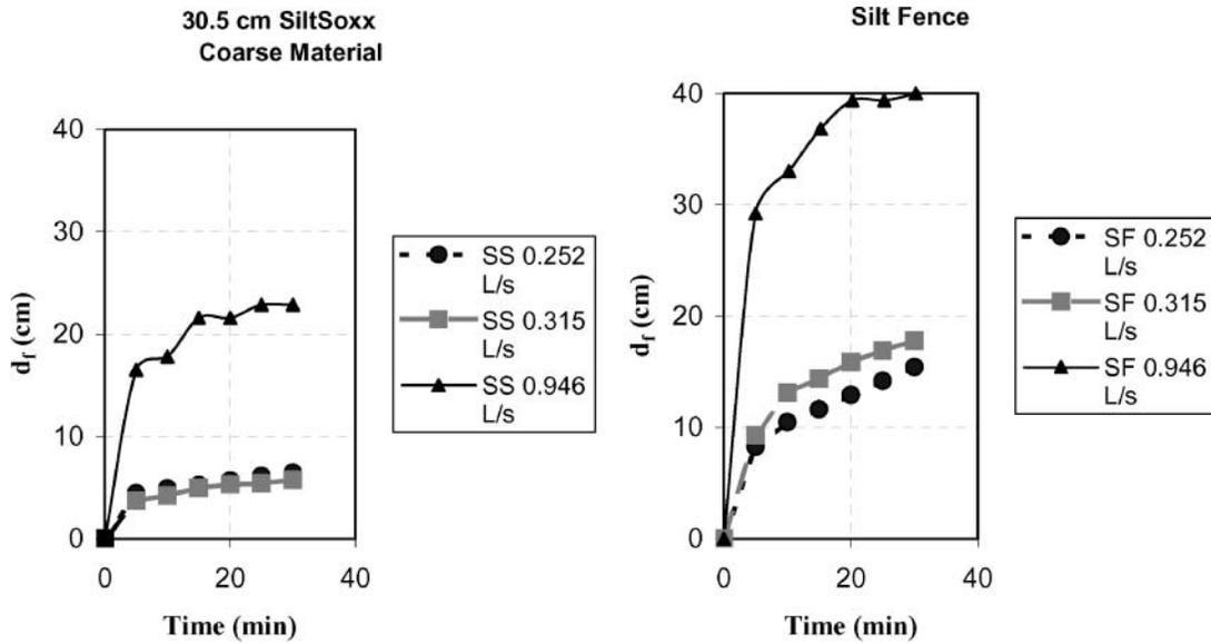
Fig. 6. Effect of time on depth of sediment-laden water retained by the 30.5-cm diam. (12 in) coarse SiltSoxx and silt fence.
