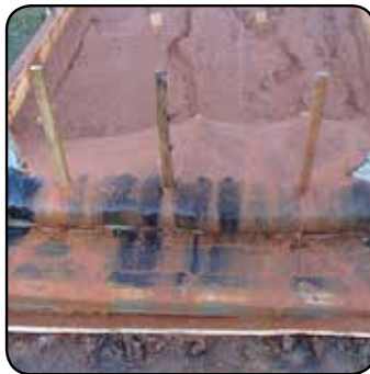
Fig. 3: 12" Off-Spec Compost Sock (66% Removal Efficiency)
