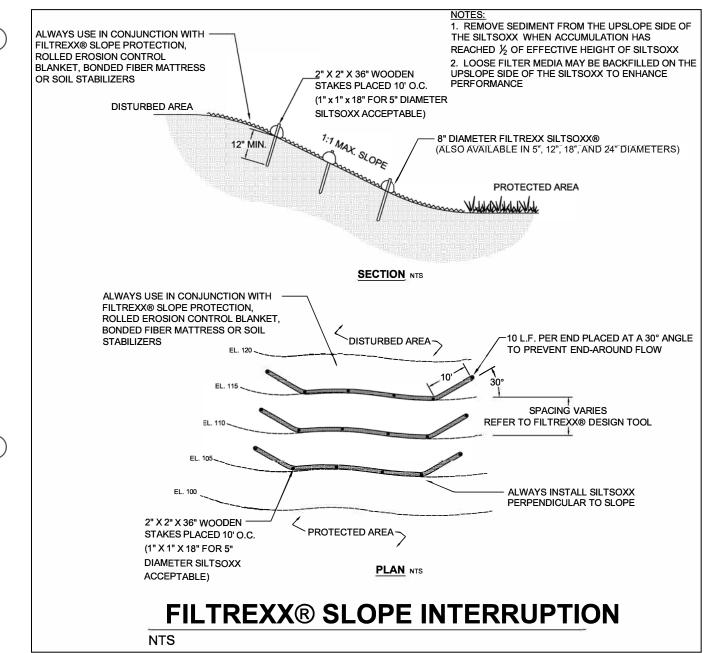
Figure 5.2. Engineering Design Drawing for Slope Interruption - Staking Details
