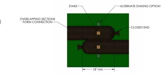
NOTES: 1. ALL MATERIAL TO MEET FILTREXX® SPECIFICATIONS. 2. SILT SOXX FILL TO MEET APPLICATION REQUIREMENTS. 3. COMPOST MATERIAL TO BE DISPERSED ON SITE, AS DETERMINED BY ENGINEER.
