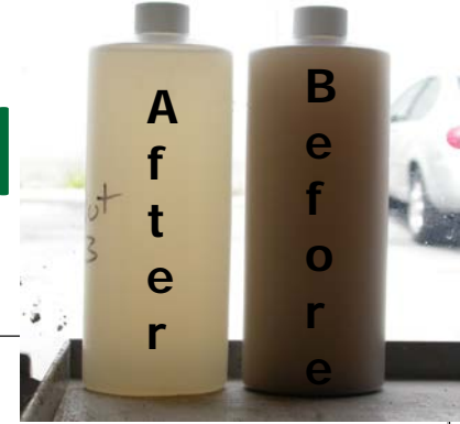
FilterSoxx Fine Sediment Removal over 30 min Runoff Event
