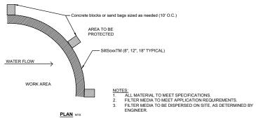
SiltSoxxTM for Sediment Control on Pavement
